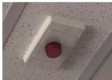
On-Air Light – Camera in Standby
