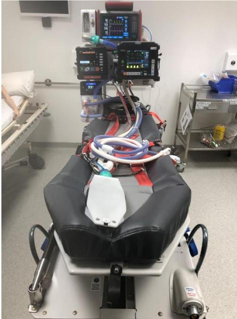
*Paediatric Life Support System – incorporating previously separate Stretcher and Bridge – NETS and Total Aerospace Solutions*
